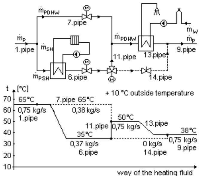
**Fig. 4.** Simplified scheme of serial connection substation with the results of simulation
