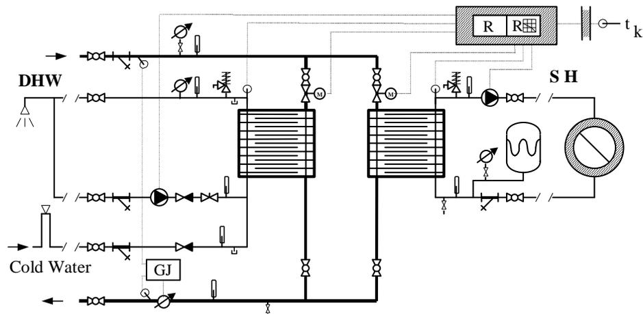
**Fig. 2.** Consumer substation with parallel connection of heat exchangers
