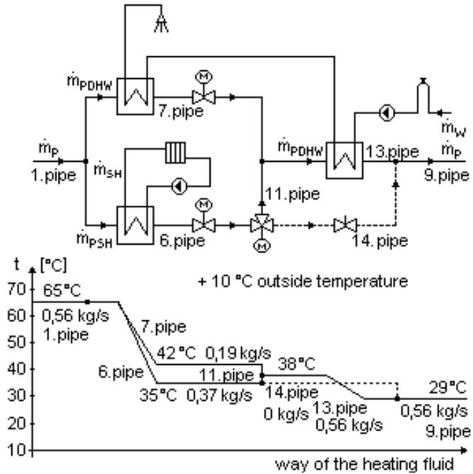
**Fig. 6.** Simplified scheme of two-step connection substation with the results of simulation
