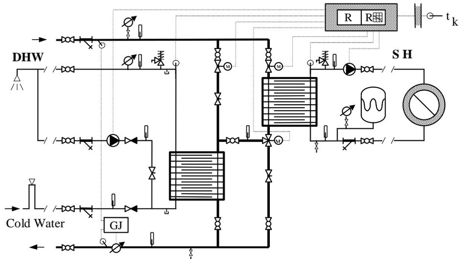
**Fig. 1.** Consumer substation with serial connection of heat exchangers
