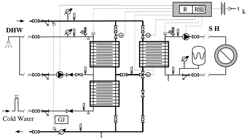
**Fig. 3.** Consumer substation with two-step connection of heat exchangers
