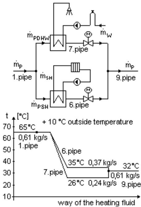
**Fig. 5.** Simplified scheme of parallel connection substation with the results of simulation
